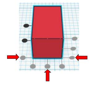
**Move** <u>Top Hinge</u> (Must be in home view for this to work!) move back in positive Y direction 3mm
