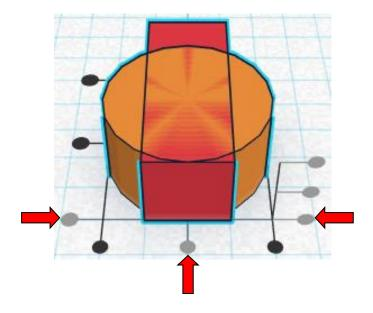
**Move** Key Hole Cylinder (Must be in home view for this to work!) move forward in negative Y direction 3mm
