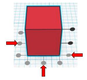
**Move** Right Hinge (Must be in home view for this to work!) move down in negative Z direction 7mm
