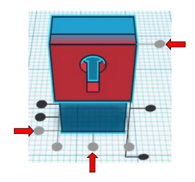
**Move** Lock (Must be in home view for this to work!) move up in positive Z direction 12mm
