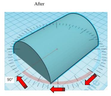
Bring in a Round Roof, located in Basic Shapes on the left 5 shapes down. From now on this will be called the **Lid Accent**
