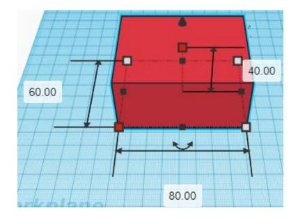
Bring in a Box, located in Basic Shapes on the left 2 shapes down. From now on this will be called the **Base Cutout**.
