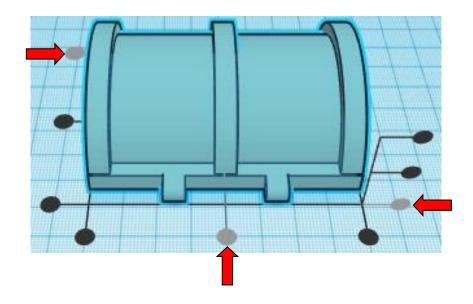
**Move** <u>Lid</u> (Must be in home view for this to work!) move forward in negative Y direction 1mm
