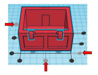
**Move** Base (Must be in home view for this to work!) move down in negative Z direction 6mm and move forward in negative Y direction 2mm
