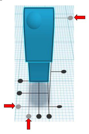
Move Right Hinge (Must be in home view for this to work!) move right in positive X direction 2mm and move forward in negative Y direction 1mm and move up in positive Z direction 1mm
