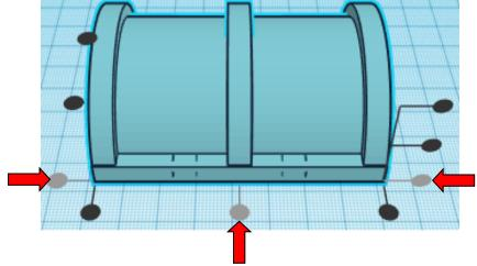
**Move** <u>Lid</u> (Must be in home view for this to work!) move back in positive Y direction 6mm
