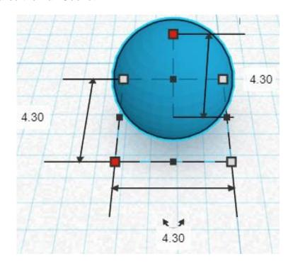
Change Ball Socket to Hole by selecting Ball Socket and typing "h".
