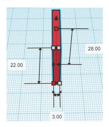
**Move** <u>Side Cutout</u> (Must be in home view for this to work!) move back in positive Y direction 26mm
