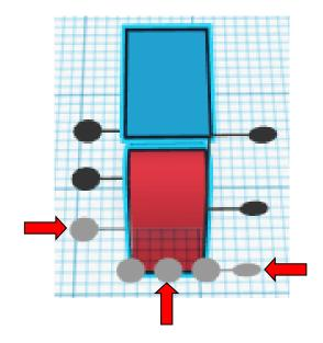
**Move** Right Hinge (Must be in home view for this to work!) move up in positive Z direction 20mm
