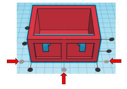
Move Bottom Hing Set (Must be in home view for this to work!) move forward in negative Y direction 6mm and move up in positive Z direction 14mm
