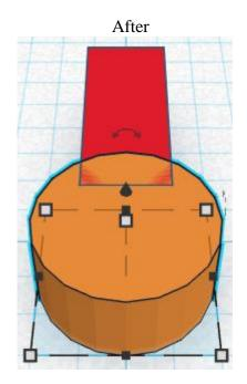
**Group** Key Hole Cylinder and Key Hole Box From now on this will be called the **Key Hole**
