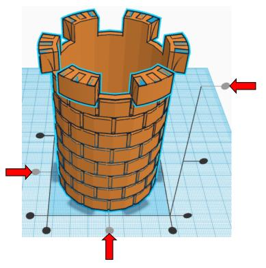
Because the <u>Full Brick Support Set</u> will be hard to select for movement, let's move the Turret instead and then we will set it back onto the workplane.
