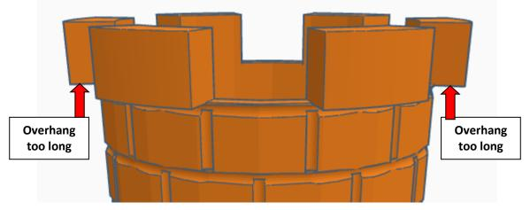
See that overhanging brick? A 3D printer can print some overhang, about 2mm - 3mm, without messing up.
