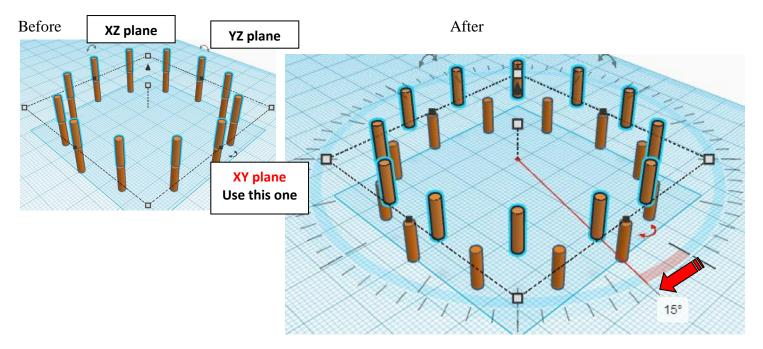
Change Double Full Cylinder Cutout Set to Hole by selecting Double Full Cylinder Cutout Set and typing "h".
