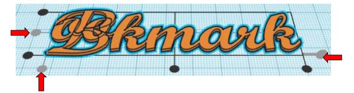
**Move** <u>B</u> (Must be in home view for this to work!) move left in negative X direction 24mm
