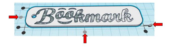
**Move** <u>Base</u> (Must be in home view for this to work!) move left in negative Y direction 3mm
