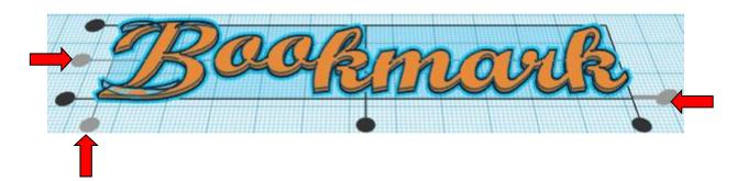
**Move** <u>Face</u> (Must be in home view for this to work!) move right in positive X direction 27mm
